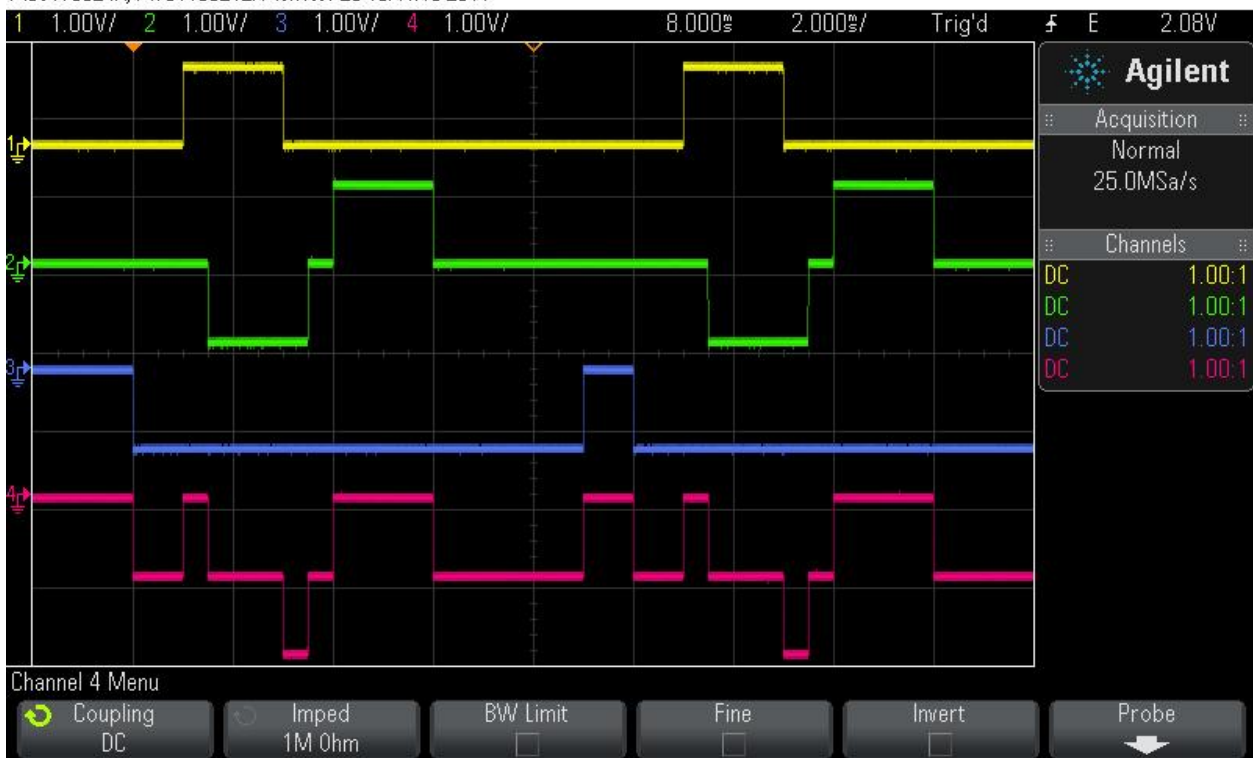
Figure 33. Examples.ams Test Program – Channel 8 Sum Out Waveforms
